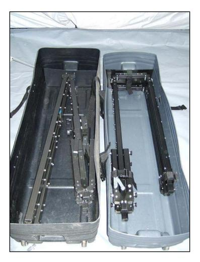
The **BlackWatch™** projector v-arm (on the left) is folded and ready to put in the case. It folds much more efficiently, and takes up less space than the old TMSS folded projector v-arm (on the right).
